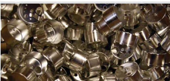
Coated part used in fuse on 60, 81 and 120mm mortar shells.
